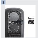
Release the old batteries by pressing the button. Remove the old batteries.
