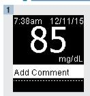
After performing a blood glucose test, the test result is displayed on the screen with Add Comment highlighted.
