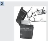
Remove a test strip from the test strip container. Close the cap tightly.
