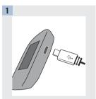
Plug the small end of the USB cable into the meter.
